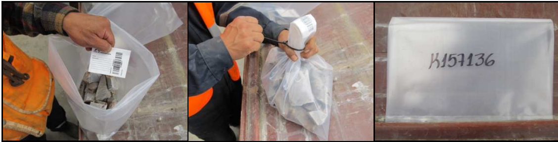
FIGURE 11-12: BAGGING SPLIT CORE INTERVALS
