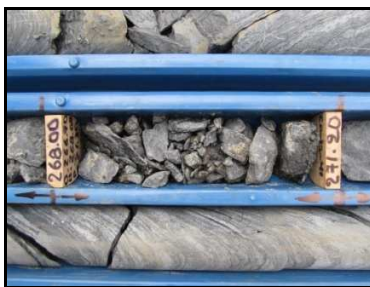
FIGURE 11-5: EXAMPLE OF SAMPLE INTERVAL WITH POOR CORE RECOVERY
