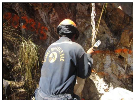
FIGURE 9-9: COLLECTING A SURFACE ROCK SAMPLE
