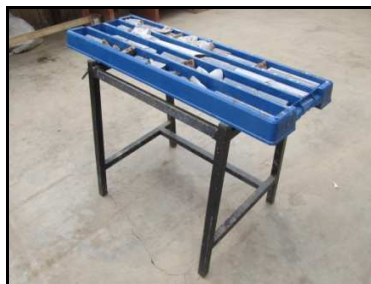
FIGURE 11-11: BOX CONTAINING CUT CORE READY FOR SAMPLING
