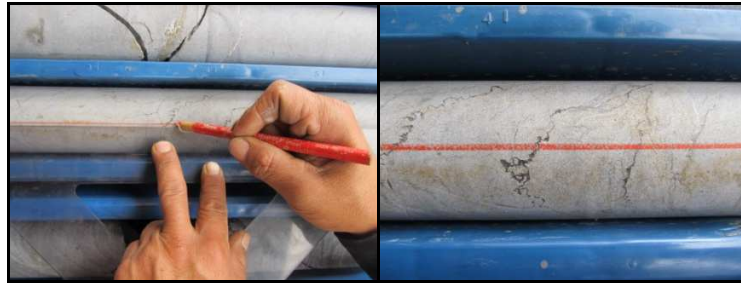
FIGURE 11-7: LINE MARKED ON CORE INTERVALS FOR CUTTING
