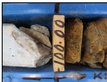
FIGURE 11-4: CORE SAMPLE MARK-UP
