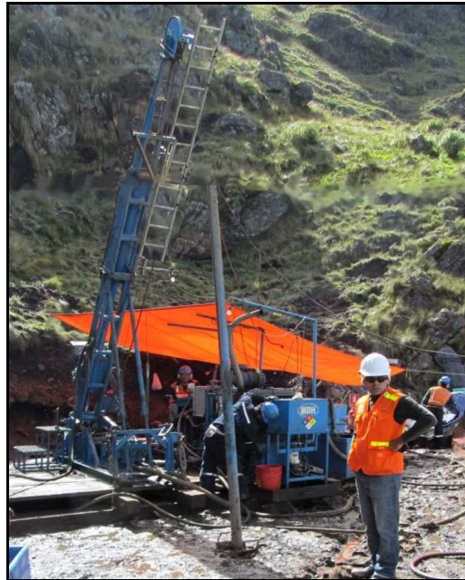
FIGURE 10-5: DIAMEC 250 DRILL RIG
