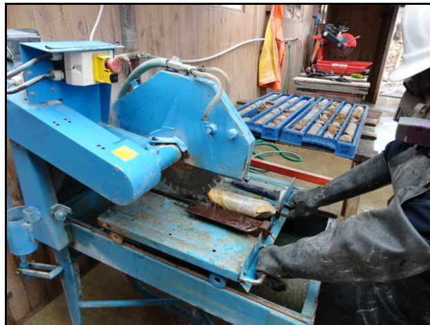
FIGURE 11-10: DIAMOND SAW USED TO SPLIT CORE SAMPLES
